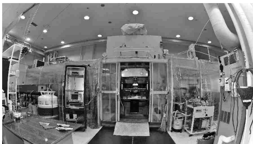
Figure 3. Horizontal single-turn coil system surrounded by measurement instruments. The single-turn coil is mounted at the center of an explosion-proof iron chamber (center of the photo). A shockwave-absorbing balloon (1 m × 1 m × 2 m, made of Kevlar synthetic fiber) is installed on the chamber's ceiling. The front access sliding doors consist of double-layered, 5-mm-thick transparent polycarbonate plates, which provide sufficient blast resistance while minimizing shockwave back-reflection toward the sample holder. These transparent doors also allow for immediate visual assessment in case of an emergency following a shot. Lasers are housed in a nylon tent booth on the left, which protects them from explosion-generated dust. To ensure signal integrity, noise-sensitive instruments are kept in a double-layered electromagnetic shield box (iron outer wall, aluminum inner wall) located next to the liquid helium container. Light transmitted through the sample is directed into the left booth, where mirrors and detectors are aligned on an optical bench. [Photograph taken by the author at ISSP, The University of Tokyo].
