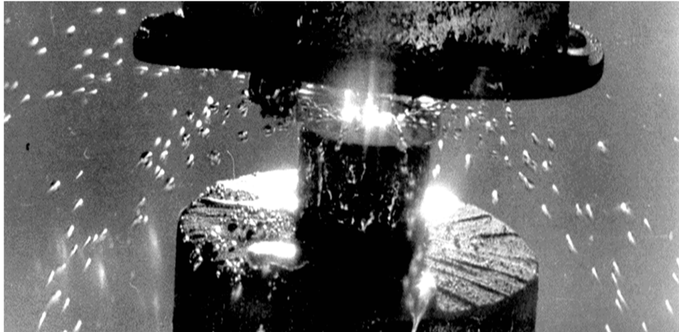
Figure 3. Electromagnetically controlled film flow disintegration in resonant regime.
