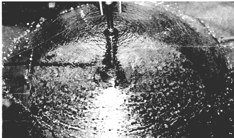
Figure 1. Thin film flow created by vertical jet due to shock on horizontal plate.
