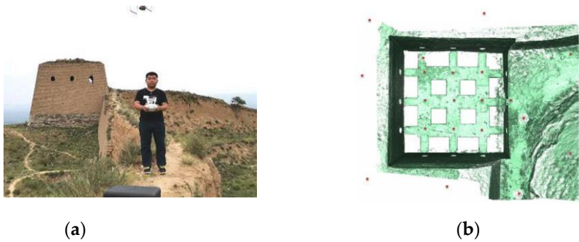
Figure 6. (a) UAV for surveying the exteriors; (b) Scanning station inside the Tower. Source: [56].
