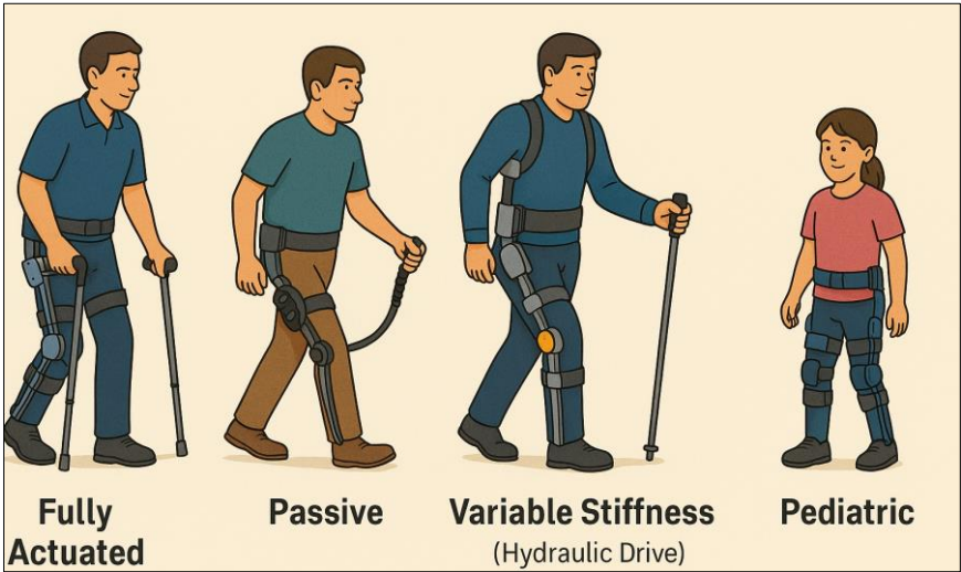
Figure 5. Hardware design and actuation strategies in lower limb exoskeletons. (1) Fully Actuated systems offering high control precision, (2) Passive designs utilizing mechanical elements like springs, (3) Variable
