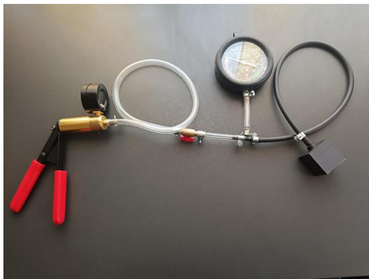
Figure 9. Prepared 3D-printed vacuum chamber for testing.
