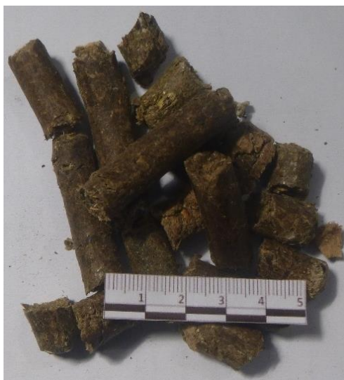
Figure 3. Prepared Waste Serving as an Alternative Fuel for Gasification.
