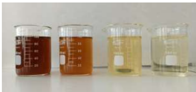
Figure 8. Efficiency of LL treatment, from the left: raw leachate, after PC, after m-IME and after m-IME/H 2 O 2 (sample 1.3).
