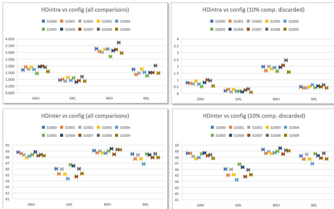
Figure 13. HDintra (top) and HDinter (bottom) values before (left) and after (right) discarding 10% of challenges for different configurations
