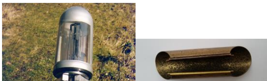
Figure 7. a Solar tracker using CuZnAl-shaped memory springs. b Details of the CuZnAl shape memory spring.
