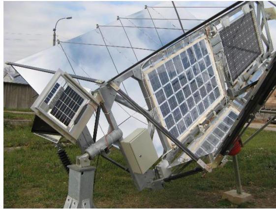
Figure 16. Pseudo parabolic concentrator with a bifacial tracking panel and mirror. The linear actuator is fixed at the bottom side of the axle (easy access).
