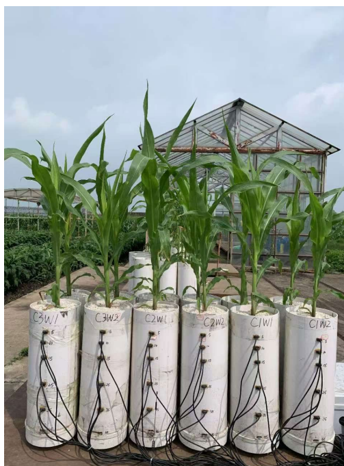
Figure 6. Experimental devices and soil water content monitoring.
