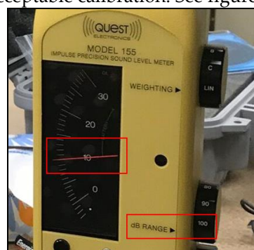
Figure 1: Sound Level Meter Calibrations
