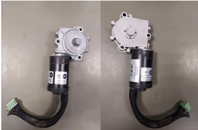
Figure 6. Brushed DC Motor with reducer which is used for design of the system.
