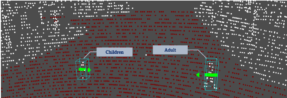
Figure 21. Pedestrian data captured by a 64 channel LiDAR (intersection).
