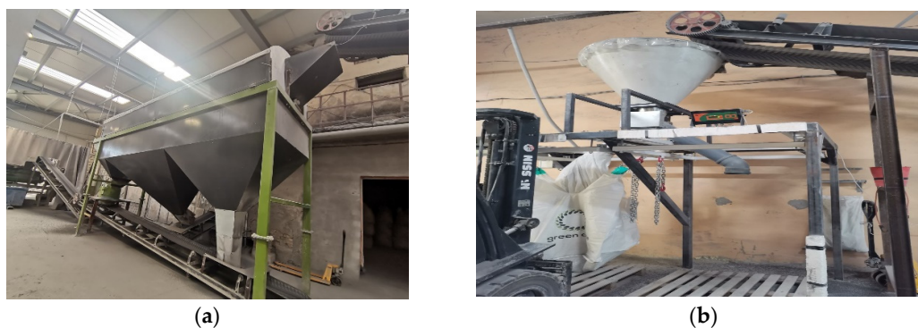
Figure 4. Delivered and constructed facilities by Green circle biotech Ltd. at the Polski Trambesh site: (a) Screening machine; (b) Packing machine.
