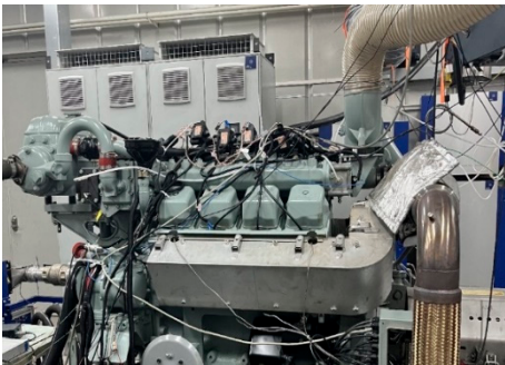
Figure 8. Methanol engine bench test setup.
