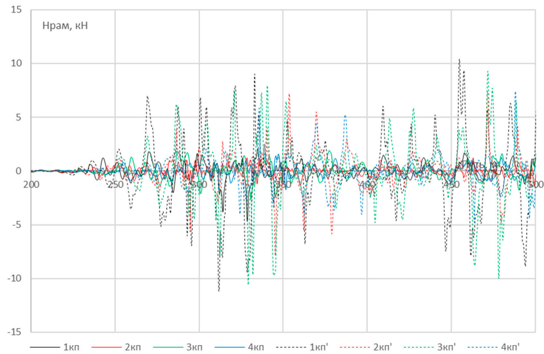
Figure 37. Oscillograms of the frame forces of the wheel pairs (wp) of the 8th car (dashed values correspond to coast down mode).
