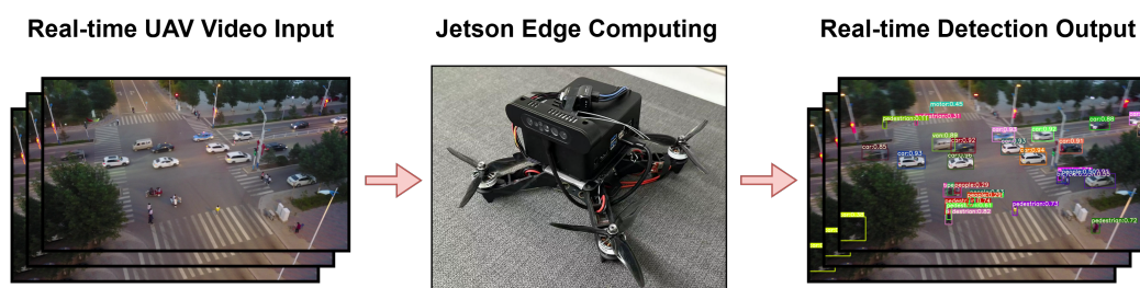
Figure 1. The end-to-end video object detection pipeline on the Jetson edge platform.
