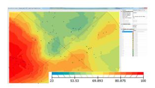
Quite a variation in attenuation values (23<attenuation<100) is seen throughout the map, resulting in increasing semi-covariance values. The stations located close together are more spatially correlated to each other than the stations located far away. In case of moving cloud day, the solar power production will be highly unpredictable in the concerned region, hence power utilities must be very cautious to manage this uncertain power with traditional power supply networks.
