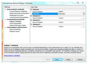
In the above interface, attenuation parameter is selected to check for spatial autocorrelation among the station. In the next window (Figure 23) select Kriging Type as Ordinary and output surface type as prediction. The Kriging/Co-Kriging method check spatial correlation between the neighboring points on map by dividing the target area into sectors of a circle.
