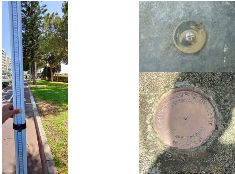
Figure 7. Invar and Leveling Benchmarks installed by Laboratory of Geodesy and Hydrographic Surveying, Cyprus University of Technology.
