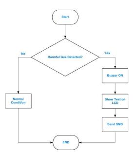
Figure 6: Flow chart of harmful gas detection section.
