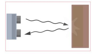
Figure 3: Diagram of the basic ultrasonic sensor operation
