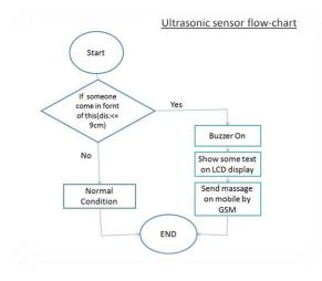
Figure 7: Flow chart of intruder's detection mechanism.
