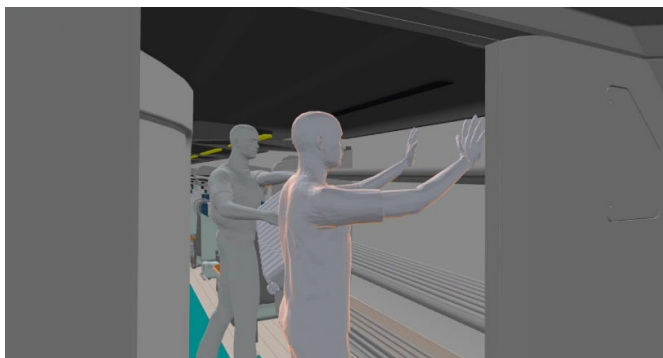
Figure 6. Evaluation of ergonomic and spatial aspects of a train interior using the VR system.
