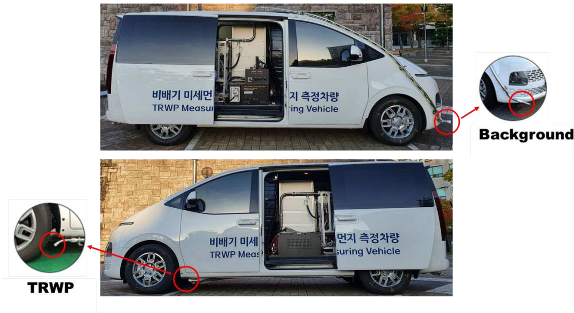
Figure 2. Photograph of the vehicle equipped with a system for measuring tire-road wear particles (TRWP). The TRWP and background sampling positions were placed in the back-side of the front left wheel and the front-side of the front right wheel for background, respectively.
