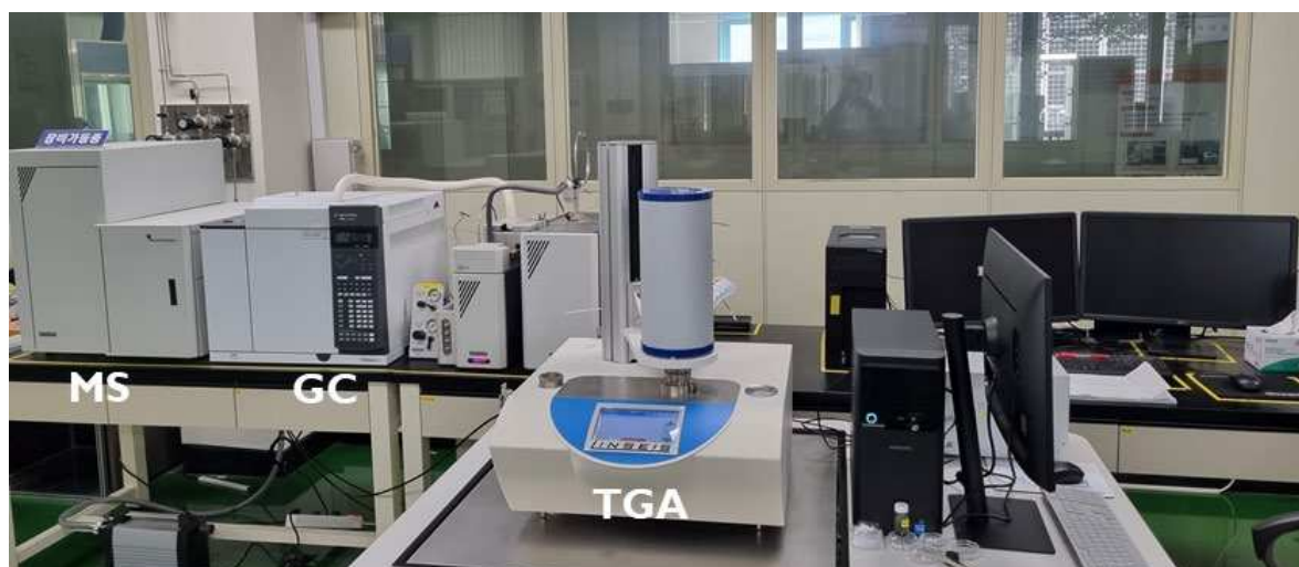
Figure 4. The photograph of thermogravimetric analyzer (TGA) connected with gas chromatography-mass spectrometer (GC-MS).
