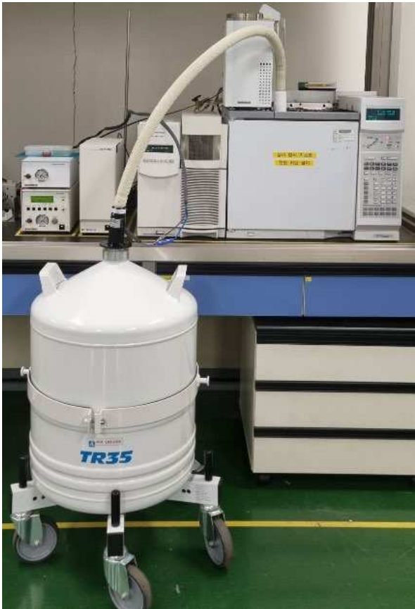
Figure 5. The photograph of pyrolyzer-GC/MS for analyzing vinylcyclohexene and dipentene in the particle samples of tire, TRWPs and background.
