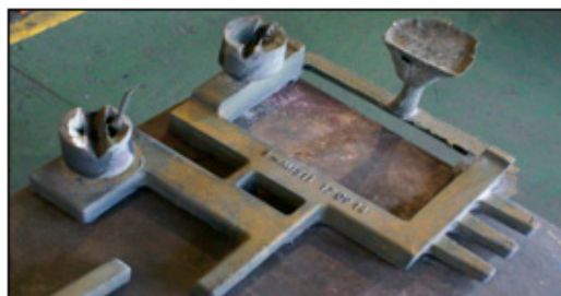
Figure 1. Experimental lattice casting component after casting shakeout process, i.e., GCW.
