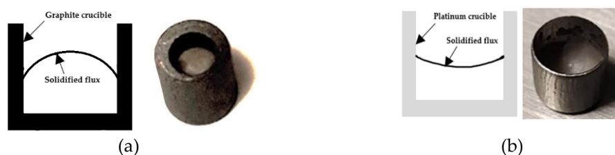
Figure 3. Schematics of the section slice of the flux-crucible appearance right after the DSC test in: (a) graphite crucible; and (b) platinum crucible.
