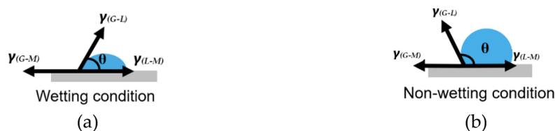
Figure 2. Schematics of (a) wetting and (b) non-wetting conditions of mold flux in contact with mold wall.
