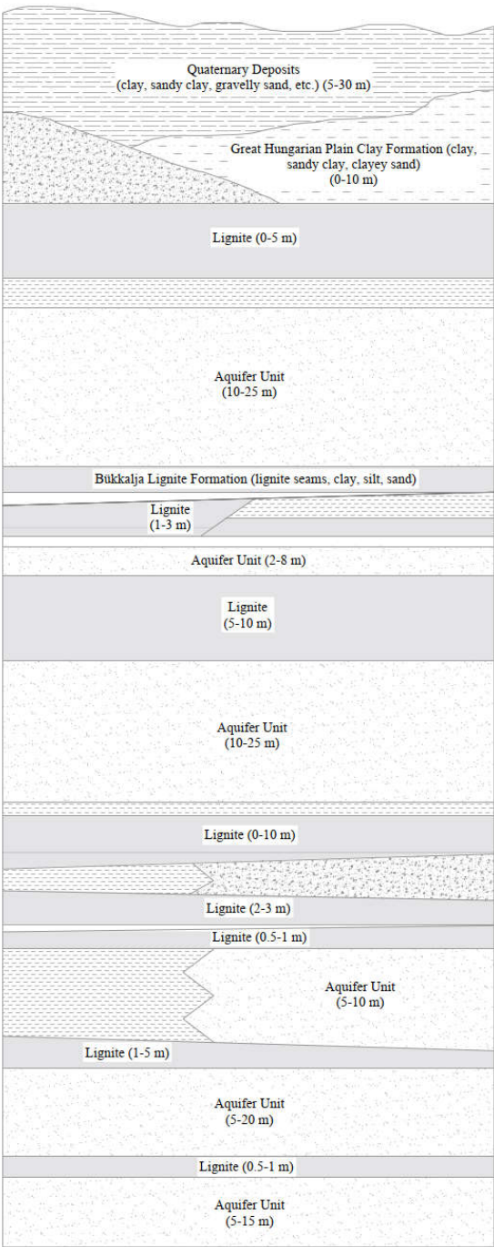
Figure 3. Geological structure of the Keleti-I mine (simplified, schematic stratigraphy) [14].
