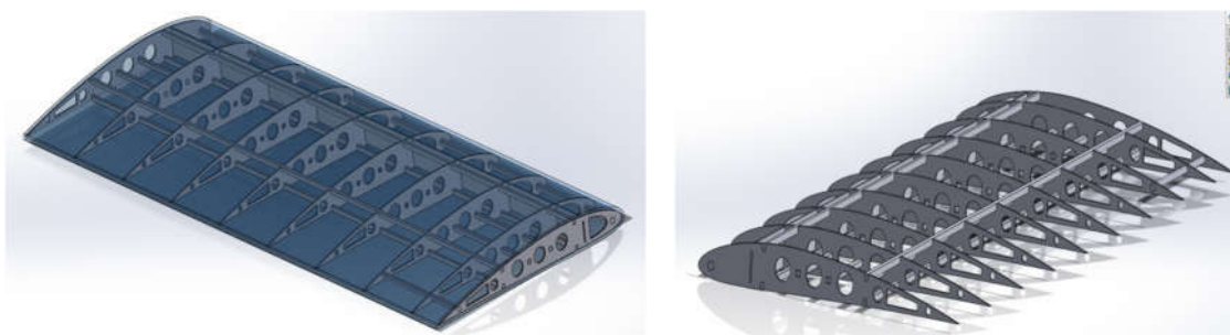
Figure 2. Wing Ribs and Internal Structures.
