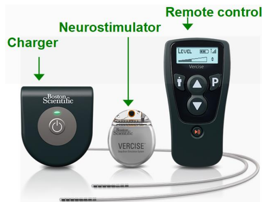
Figure 3. Commercial DBS system from the company Boston Scientific (adapted from [34]).
