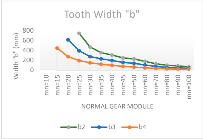
Figure 6. Tooth width and normal gear module.
