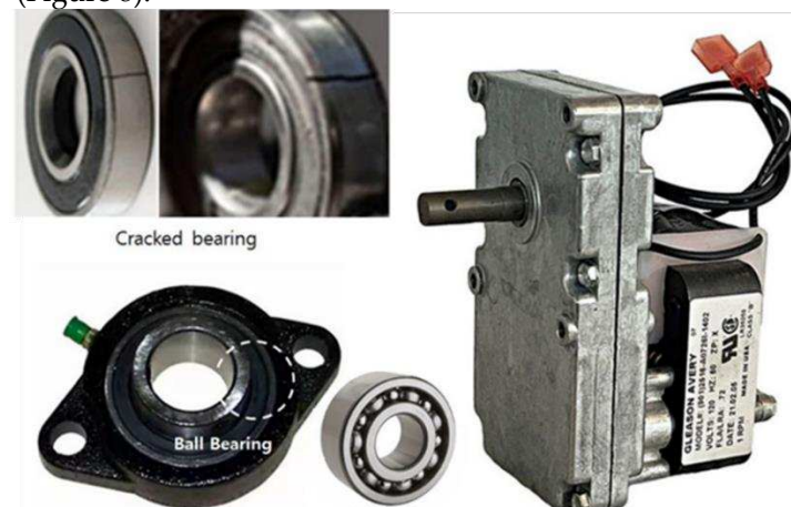
Figure 8. Failed auger motor in the market.
