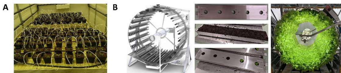
Figure 1. Representation of the control cultivation system (A) (CT lettuces) and the rotational cultivation system Gigrow® from Futura Gaïa Technology (B) (ROT lettuces). In the rotational cultivation system, plants were grown in stainless steel trays containing potting soil similar to the control.
