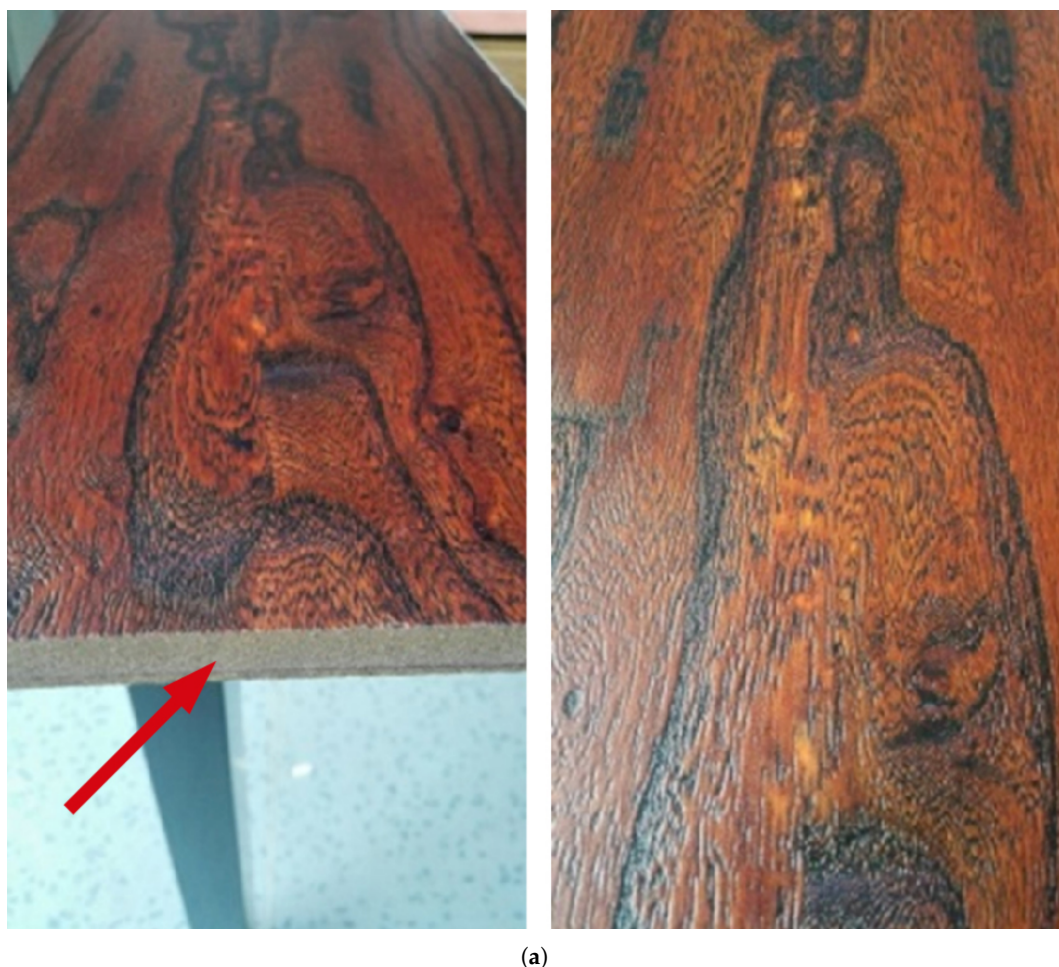
Figure 11. 3D printing an elm texture onto MDF is a direct-to-substrate additive manufacturing technique [186].
