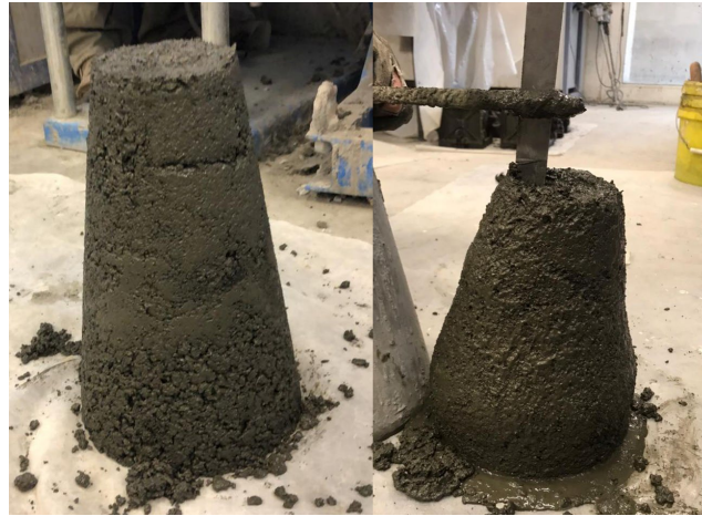
Figure 2. Slump test of fresh concrete for mixes 8 and 3.
