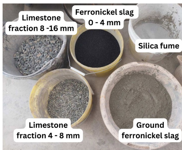
Figure 1. Dry components of ferronickel slag alkali activated concrete.
