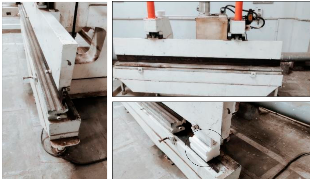
Figure 7. Shows the tooling setup for V-bending operation.
