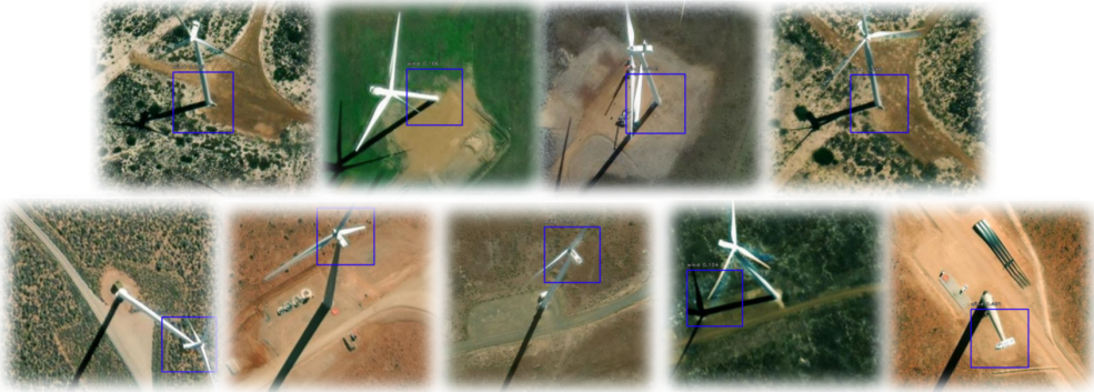
Figure 8. True positive examples from the application using the Bing images are presented as follows. The upper row displays instances featuring clearly visible and accurately identified wind turbines, where the centroid of the regression boxes serves as the base of the tower. The bottom row, shows correctly identified wind turbines, with less accurate regressive delineation in the images.
