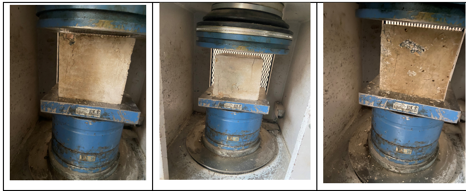
Figure 9. Fractured specimens of hardened concrete after compressive strength test.
