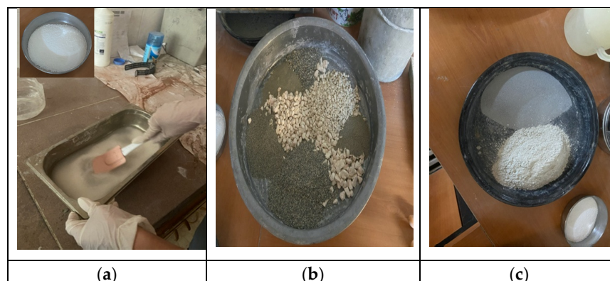
Figure 3. Mixing and curing stages of MS based OPGC a. dissolving of solid activator in the water, b. coarse and fine aggregates, c. MS (up) and GGBS (bottom) used for experiment.
