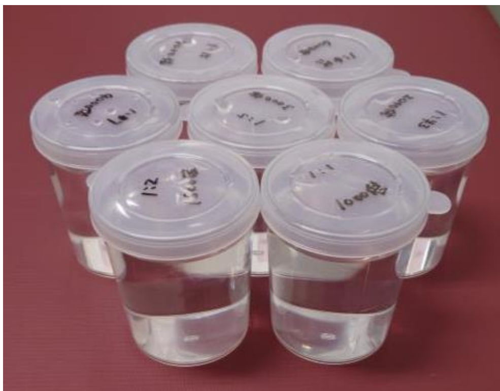
Figure 1. The photograph of phantoms. Seven phantoms were made by mixing Gd-DOTA and water and sealing them in polypropylene cylinder-shaped containers (diameter, 6 cm; height, 8 cm).
