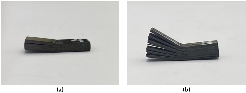
Figure 17. Short-beam shear specimens after ILSS testing: (a) virgin laminate; (b) recycled laminate.
