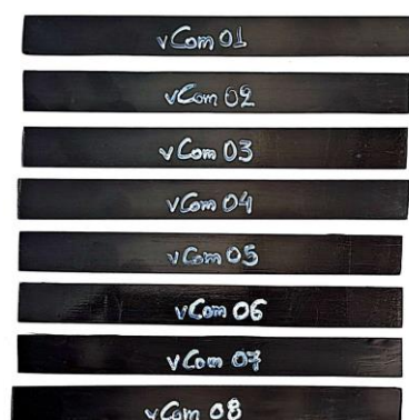
Figure 7. The compression specimens which were used for compressive testing.
