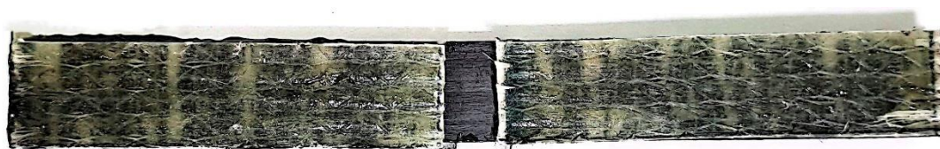
Figure 8. A compression specimen with end tabs.
