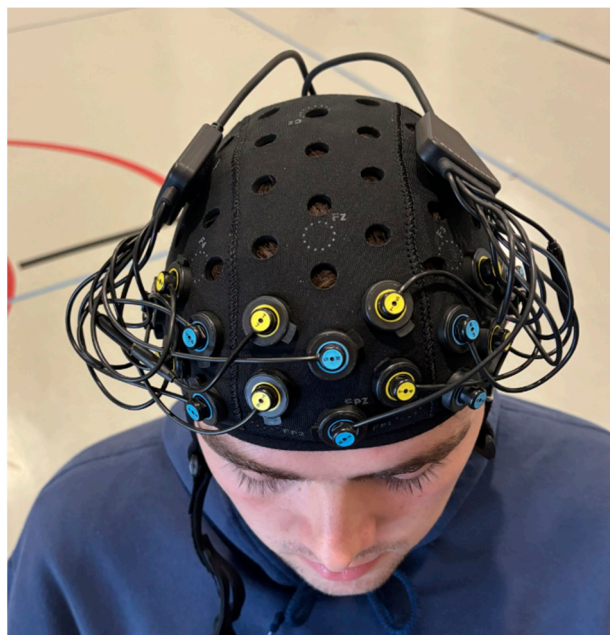
Figure 2. fNIRS system and prefrontal optode montage.
