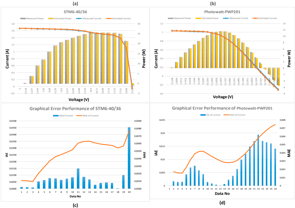
Figure 11. Performance Comparison I-V, P-V and Error Metrics for Each Data Point; (a), (c) STM6-40/36 and (b), (d) Photowatt-PWP201.
