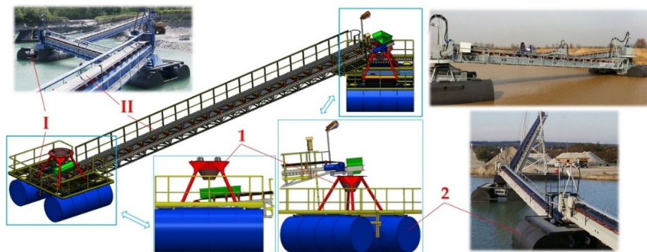
Figure 1. Floating belt conveyor. I – floating body, II – belt conveyor, 1 – turntable structure, 2 – float of a circular cross-section.
