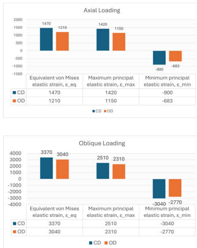
Figure 2. Mean peak peri-implant cortical bone elastic strain under (A) axial and (B) oblique loading for CD and OD models. Values are reported in microstrain ( \mu\epsilon ); negative values indicate compressive strain. For each outcome, the mean of the 10 nodes representing the high-tail response (as defined in Table 2) was computed.
