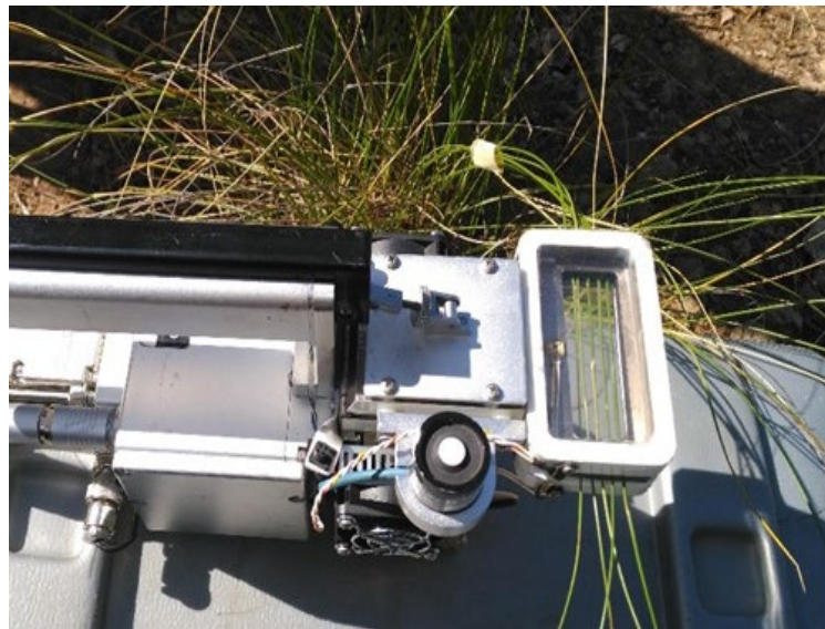
Figure 2. Measurement of transpiration in Stipa tenacissima L. leaves using the LI-6400XT portable equipment. The setup involved the use of the 6400-07 Needle Chamber, specifically designed for needle-like leaves. The sample consisted of 5 segments of leaves.
