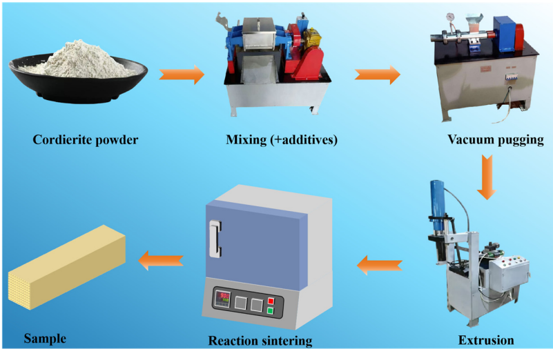
Figure 1. Schematic of extrusion molding method for fabrication of honeycomb shaped cordierite ceramics.
