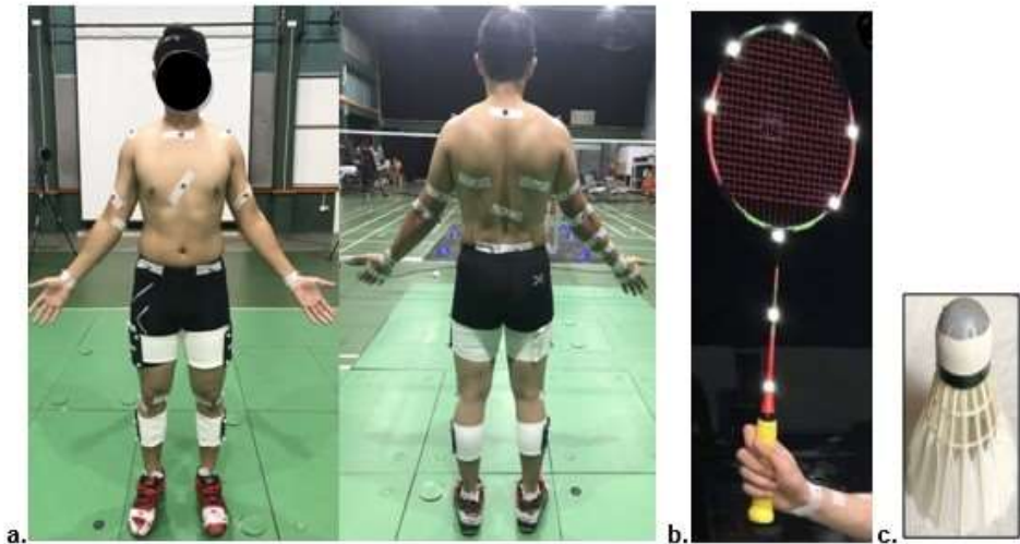
Figure 2. Marker placement on a) the participant, b) the racket c) the shuttle tip.
