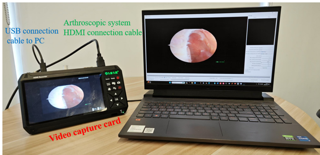
Figure 12. Video capture system setup for real-time arthroscopic visualization.
