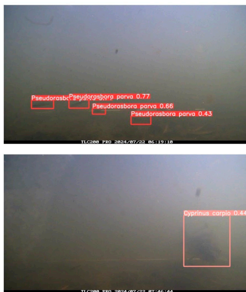
Figure 4. Examples of successful detection during inference. All the objects were correctly identified with a confidence threshold of 0.427 and an IoU threshold of 0.50.
