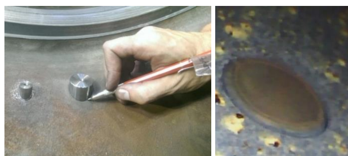
Figure 4. Left: Individual adaptation of the sensor to the respective measuring position. Right: Boroscopic picture of the inside of the casing of the steam turbine after installation. The sensors were flush-mounted with the surface of the complex internal geometry. The light-coloured particles show corrosion effects in form of rust.
