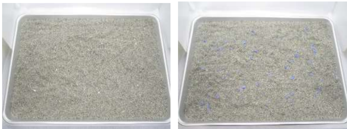
(a) White PP (Option 4; 1,000 mg-MPs/m 2 -sand) (b) Blue PP (Option 8; 20,000 mg-MPs/m 2 -sand)
