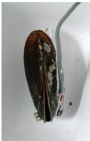
Figure 2. Valvometry sensor attached to the shell of a mussel in a lab setup: magnet (right valve) and Hall effect sensor (left valve).
