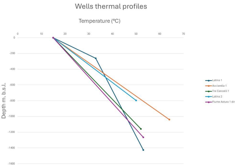
Figure 11. Geothermal well profiles Acciarella 1 and Latina 2 wells are interpreted to be drilled just above an intra reservoir convective cycle. Latina 1, Tre Cancelli 1 and Fiume Astura 1 Wells are interpreted to have a purely conductive geothermal gradient. .
